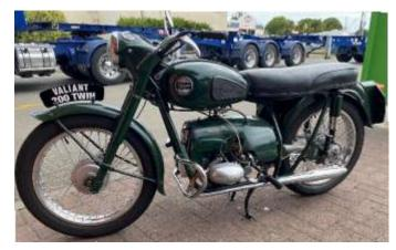
I obtained the bike from Mark Brown in Nelson last year who had the bike for 28+ years before he proceeded to go about restoring the mechanics. It has been re-bored, new pistons and valve guides, replacement rims and tyres and converted to 12volt electronic ignition. The paint work is still as original, as is the rest of the bike. have an extensive paperwork trail from Mark that would go with the bike.
