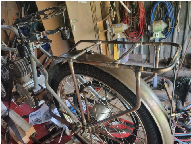
Carrier and rear guard secured
