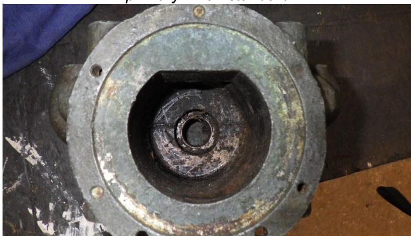
The Cambox main chamber, right side end view, shows that there are no drains, so oil only gets out via the bearing at the end, or flicked out by the action of cams through the holes in the top.
