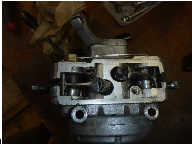
Rockers showing how oil leaves the main cam chamber through holes in the top where the rockers run on the cams
