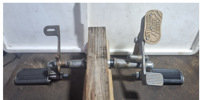
Footrests with brake and clutch pedals
