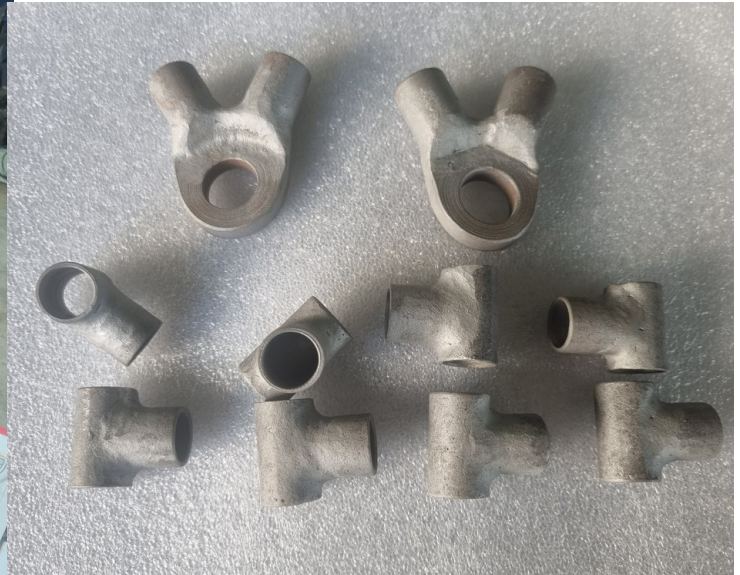
Special sockets to join the tubes of the carrier
