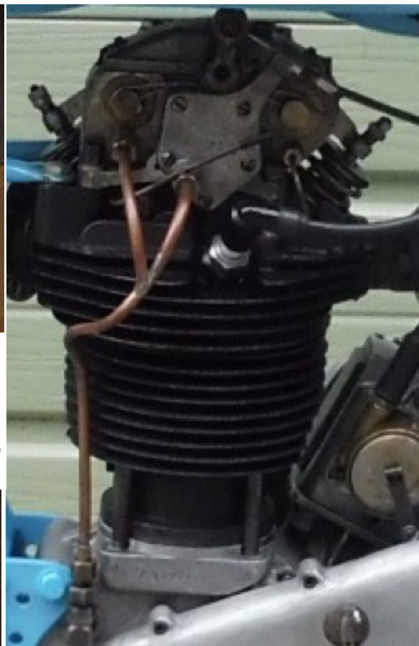
cambox drain pipes
